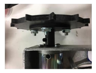
Now mount the motor into the chassis. Notice the setscrew in the shaft of the wheel. Be sure to get it aligned with the flat spot of the motor shaft. This is very important. Use Loctite to keep it from backing out during operation.
