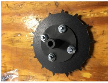
Assemble the wheels. From the picture you can see how we assembled the drive wheels first with the nuts on the inside. There is also a set screw on the side of the shaft that goes into the motor shaft.
