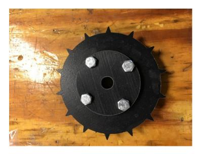
The idler wheels are assembled as shown. After this insert the bearings on each side of the wheel.
